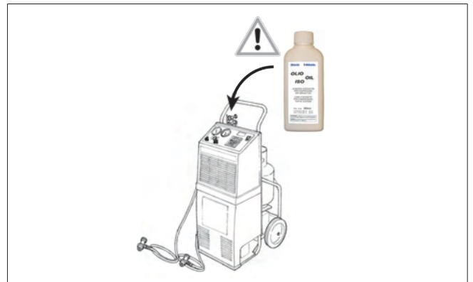
Fig. 15 Add the correct quantity of lubricant
