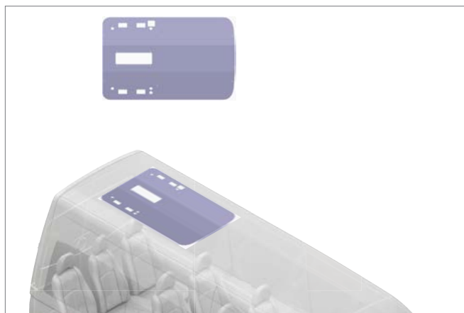
Fig. 04: Align drilling template
