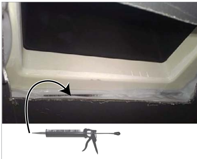
Fig. 15: Apply Sikaflex from inside the vehicle
