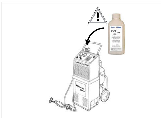
Fig. 25: Add the correct quantity of lubricant
